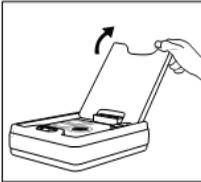
1. NT-381: Heart+ResQ™ turns on automatically when cover is opened by pushing the lower part of the cover.
